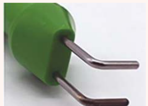
L shaped 10 mm gap contact electrode used for the electroporation
